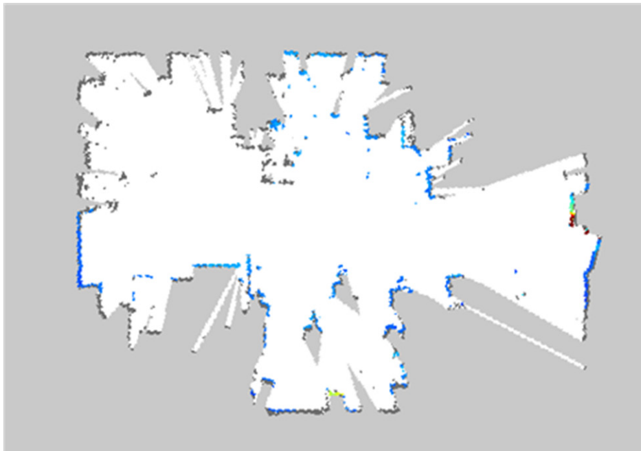
Figure c—Discrete metric map, showing the interior of a furnished room. The grey level of each cell represents how likely it is to be free space. White means certainly free , black means certainly occupied , and mid-grey means unknown . In this example, colored cells (blue-yellow-red) also represent occupied space , and additionally store the temperature of the surface, as measured by a thermal camera.
