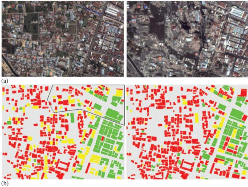
Figure 5-11. (a) Portion of bitemporal images of Banda Aceh, Indonesia region, which was taken (left) before and (right) after the 2004 Indian Ocean Tsunami, (b) training/validation input data (left), predictive damage map (right) (red: major damage, yellow: moderate damage, green: minor or no damage).
