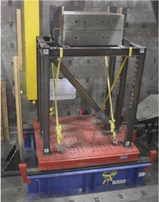
Figure 6-37. Braced frame using a Quaketek friction damper. Source: F. M. Tehrani, an experimental shake table study photo (Couch 2020).
