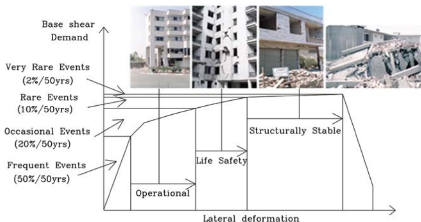
Figure 6-1. A schematic view of selecting a performance level.
